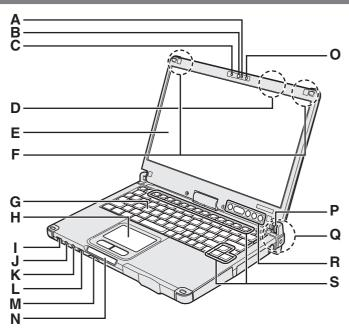
This computer contains a magnet and magnetic products at the locations circled in the illustration at right. Avoid leaving metallic object or magnetic media in contact with these areas.
