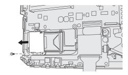
10.Remove the connectors on the built-in bridge battery.
