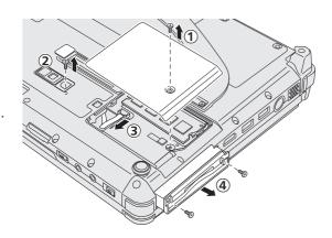
4. Remove the screws (10), and then remove the hand strap and covers (2).
