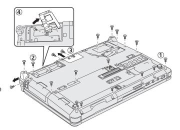
6. Turn over the computer, and open the display. Rotate the display as shown, and remove the screws (5).
